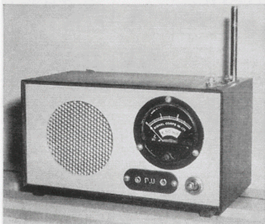
Front view of VU2JN's a.m. and c.w. transmitter.
