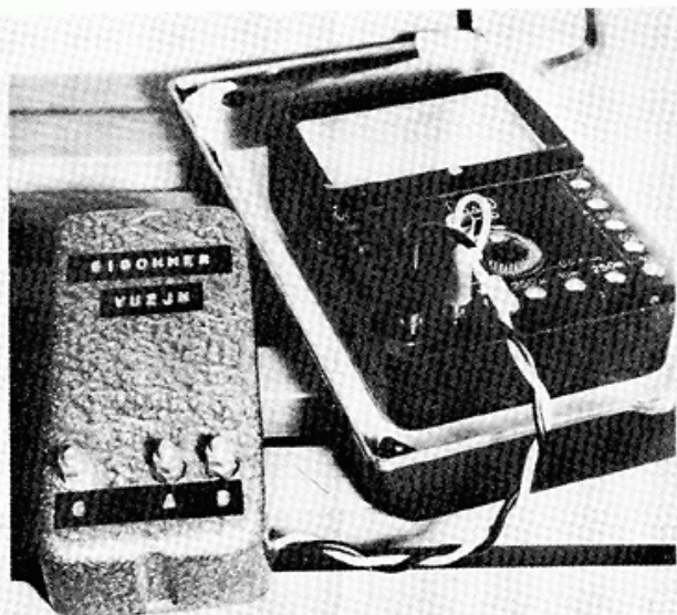
The Gigohmer connected to the author's inexpensive multi-meter. Note that terminals A and B simply pass through holes in the aluminum box.
