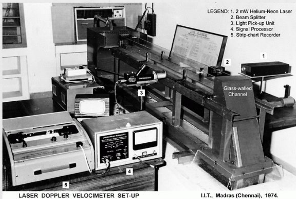
FIG.3. LASER DOPPLER VELOCIMETER SET-UP
